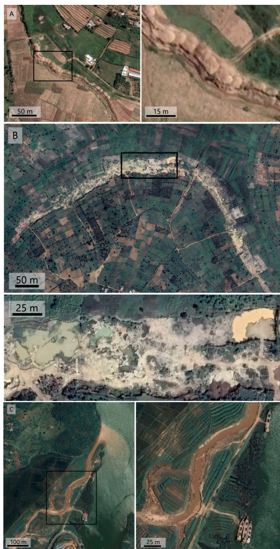
Fig. 2. Examples of sand mining. Black boxes indicate close-up of each site. A: In-stream river mining. The width of the river is less than 1 m wide, and piles of sediment are visible along the river bank near Runda, 20 km east of Kigali, Rwanda. B: Inland mining in farmfield in Nyamata, 60 km South of Kigali, Rwanda. Mining activities leave behind shallow pits, which after precipitation events get filled with water. C: In-stream river mining in the downstream part of the river running into Lake Kivu. Sediment is deposited in barges in the south-eastern part of the lake, which borders Rwanda and Democratic Republic of Congo. Barges are 45 m long, 8 m wide. All imagery is provided by Google Earth.
